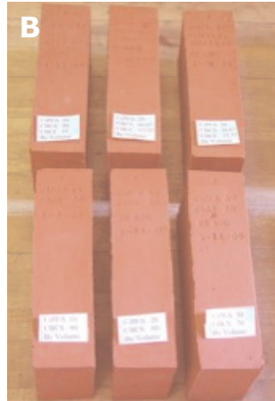
Mold-pressed paving bricks produced at the Illinois State Geological Survey bench-scale facility before (A) and after firing (B).
