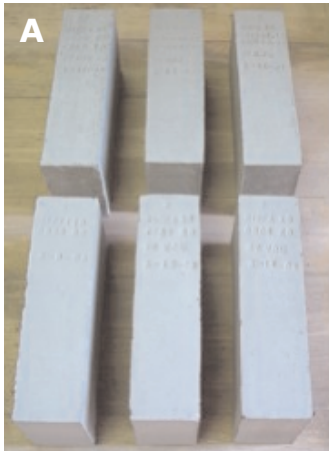
Mold-pressed paving bricks produced at the Illinois State Geological Survey bench-scale facility before (A) and after firing (B).
