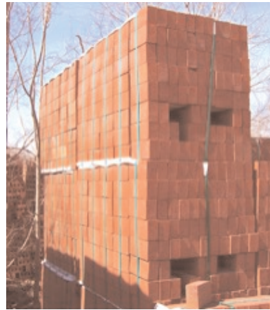
Two thousand paving bricks with fly ash from commercial scale-up production (Run II).
